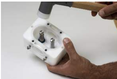
Fig. 12: Knock out the shaft
