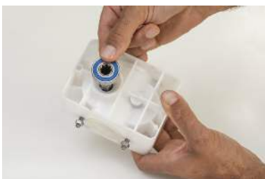
Fig. 15: Inserting the shaft
