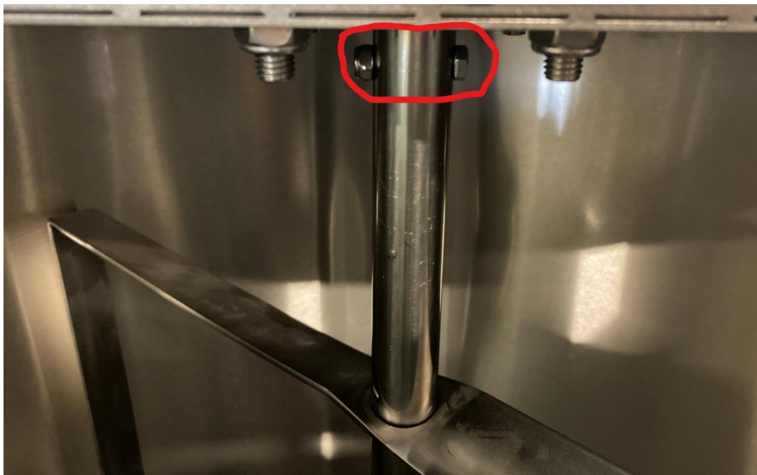
Figure 6. Whisk shaft overload protection bolt M6x30 stainless steel bolt and M6 nut.
