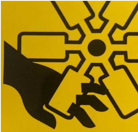
Rotating parts / risk of being trapped
