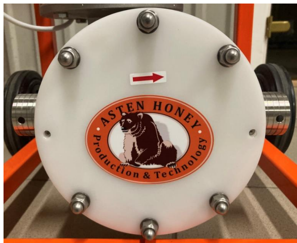
Pumping direction with red arrow
